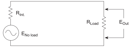
Fig. 1. Equivalent output circuit.
