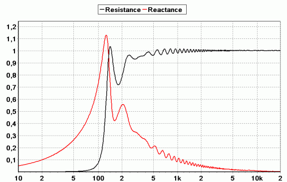
Figure 19: Throat impedance of a traxtrix horn.
